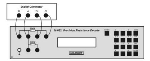
Recommended connection of standard ohm-meter for calibration points R27 to R35 (terminals R2W):
